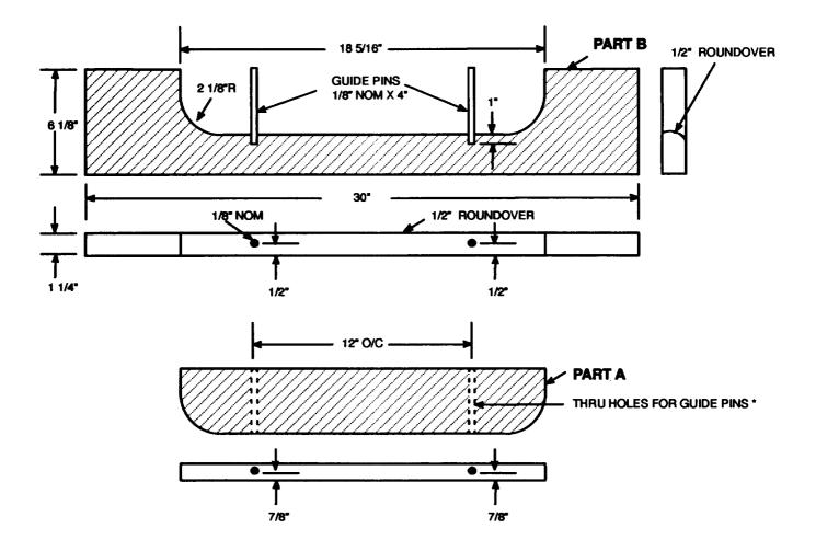
FORMER W/INSERT USEDTO FORM EXHAUST DUCT EXTENSION/ STIFFENER MAKE FROM MATERIAL --1 1/4" X 36" X 36" PHENOLIC SHEET, NSN 9330-00-290-1668
